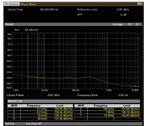
Phase Noise Measurement Low Phase Noise Performance MS2840A-066 Off 150 MHz Measurement Frequency, Preamp Off
